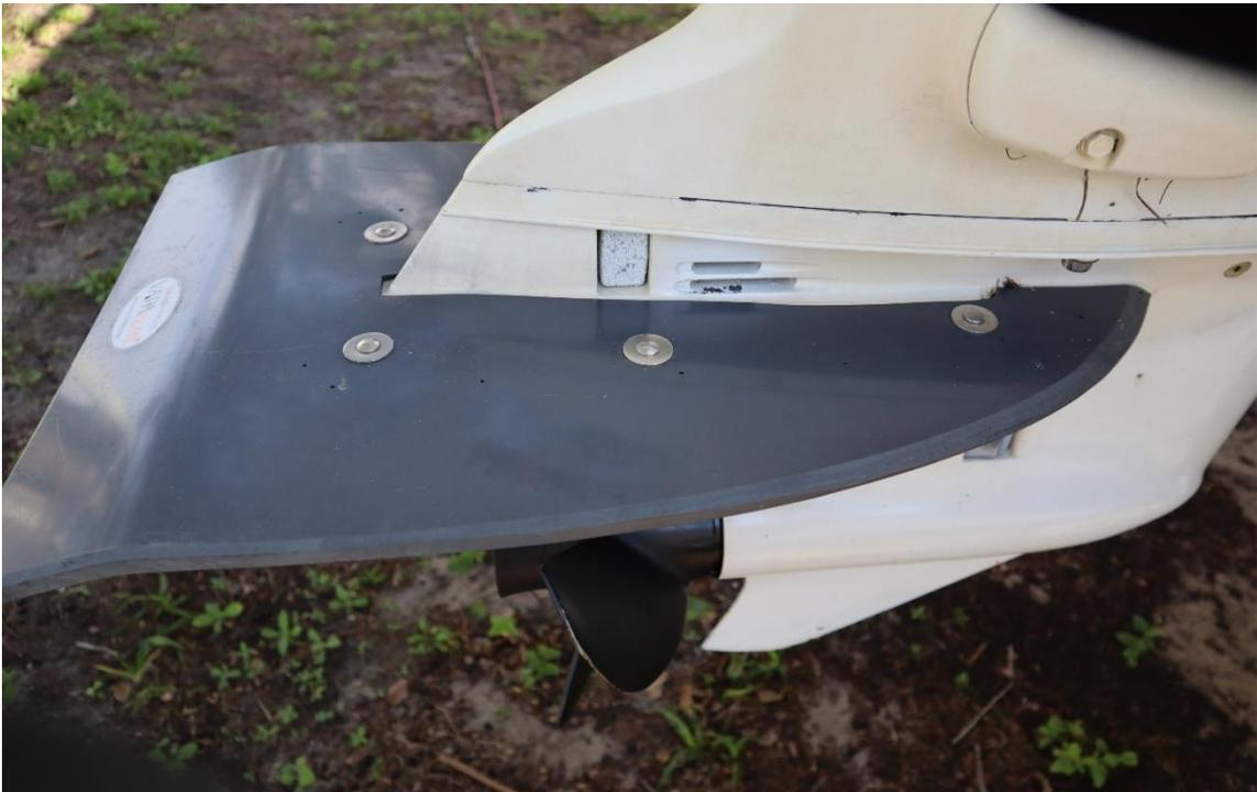
**Above install was completed on 75 Hp Etech and has 7 bolts total, as middle aft is missing. 90 Hp-150Hp we recommend using 9 total bolts as shown in diagram. 150-350Hp we recommend using 11 total bolts as shown in 2<sup>nd</sup> diagram.**
